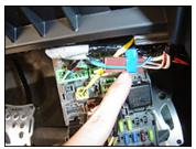
Plug the remaining 1-pin connector from the switch harness into this 1-pin connector. Then secure the 1-pin connector to the main
