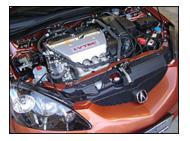
Remove the power steering reservoir and continue routing the fog light 2-pin connector behind the right headlight along the main harness, then hang it down the front bumper through the hole at the rear of the right headlight:
