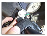
Remove the retainer clip from the 16-pin connector. You'll probably need a thin flat head screw driver to pop the retainer out:
