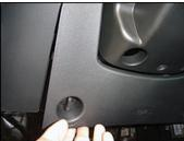
Next, locate the driver's side dashboard undercover and turn the knob counterclockwise. Pull the cover down towards the pedal to unhook the retainer clip, then pull the cover towards the driver seat to remove the cover from its holder:
