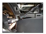
21. On manual transmission vehicles, hold the silver collar beneath the shift knob and pull down to remove it from the shift knob re-tainers, then remove the shift knob by turning it counterclockwise.
