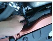
Secure the fog light harness to the hole in the bulkhead upper frame with the wire tie with clip.
