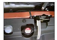
Pull out the right front-inner fender and remove the vehicle ground bolt from the right front side frame. Secure the ground terminal of the fog light harness with this ground bolt:
