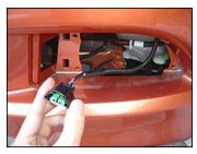
Route the fog light harness 2-pin connector (long end) along the vehicle harness behind the left headlight and inside the bulkhead upper frame toward the right (passenger's) side of the vehicle:
