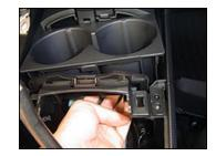
24. Inside the center console, remove two screws located midway across.
