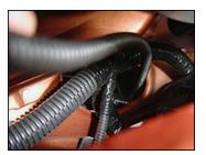
11. Secure the fog light harness 1-pin connector connected behind the left headlight to the main harness with one wire tie:
