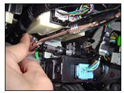
38. Plug the switch harness 4-pin connector into the relay:
