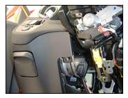
30. Route the terminal end of the switch harness to the top of the steering column, along the main harness. Above the steering column, disconnect the 16-pin connectors. This connector is located right behind the light switch:
