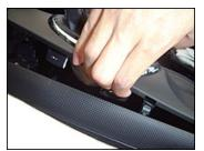
22. Remove the two self-tapping screws that fastens the center console to the dash:
