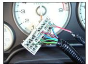
Snap the connector retainer back in place (make sure you hear it snap), then reconnect the 16-pin connector back to its original location.
