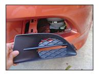
Remove the two self-tapping screws and one clip, then pull the inner fender out towards the wheel, so the interior is exposed.
