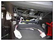
34. At the center console opening, unplug the vehicle's 12-pin connector:
