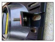
Attach outer fog light trim onto the hook on the bumper and screw it into place by tightening the  $5 \times 16$  mm washer-screw:
