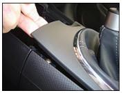
Then carefully continue lifting up the center console trim along the edges, alternating between the left edge and right edge:
