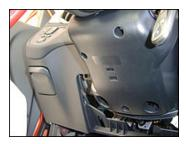
and remove the steering column upper and lower covers (six retaining tabs) by pull them apart:
