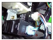
39. Pull the switch harness 5-pin connector out through the instrument panel and plug it into the rear of the fog light switch. Install the switch into the instrument panel with the led indicator facing up:
