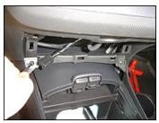
Then remove the two screws at the rear of the console. You will need to move the front seats up and hop onto the backseats to remove these two screws:
