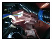
Route the fog light harness 2-pin connector (short end) down into the front bumper through the same hole as the windshield washer tank:
