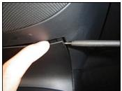
Carefully work your way around the edges, pulling the cover outward and removing them from the clip holders.
