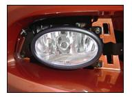
17. Insert one 5 x 16 mm washer-screw into the hole in the fog light trim in the position shown, and secure the trim with one lock washer from the reverse side:
