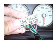
32. Insert the terminal connector from the switch harness into the 16-pin connector in the location shown:
