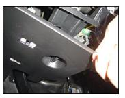
20. Pull the center cover towards you to release one retaining tab and six clips. This is easier said than done, especially if you are worried about breaking parts and panels. If you have nails, pry off the indentation on the edges. If you do not have nails, then use a very thin flathead screw driver:
