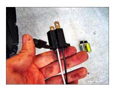
16. Close the retainer shut and snap it into place, then plug it into the stock harness. The white wire should feed into the red/yel wire; while the black wires should feed into each other:
