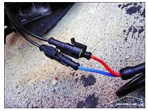
20. Plug the ignitor into the ballast and then the power harness into the ballast:
