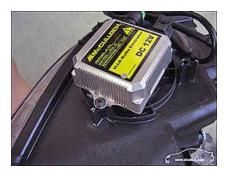
24. Next, use the included double-sided tape to secure the ignitor underneath the headlight, next to the ballast:
