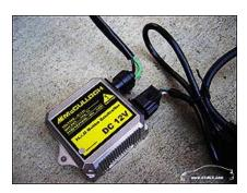
21. Repeat for the opposite headlight. Once all wires are plugged in, take the main HID wire harness and locate a red wire and a black wire. Connect the red wire to the (+) terminal of your battery and the black wire to the (-) terminal of your battery (or any part of your RSX's chassis).
