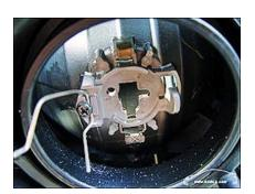
18. X-clip with HID bulb secured in place:
