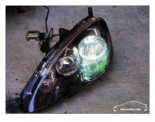
23. The ballasts are mounted them underneath each headlight. The bottom of the headlights have three protruding holes. Align one of the mounting holes of the ballast to one of these protruding holes and secure with a self-tapping screw:
