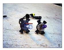
The circular indentation locks into the corresponding holes in the headlight:
