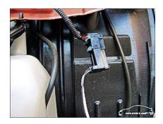
17. Next, insert the HID bulb into the x-clip and rotate it around until the two circular indentation resembles the picture below:
