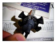
Rotate the bulb around and ensure that it fits snuggly. Once you've passed this test, it's time to connect the kit:
