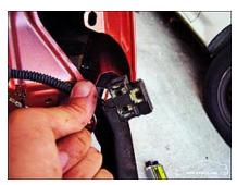
15. Noting the position of the polarity, insert the black and white wires into the empty plug:
