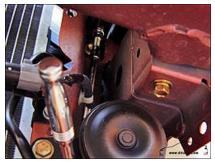
With the necessary screws and bolts removed, lift up the headlight and pull it towards you
