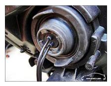
19. Next, take the wires from the HID bulb and plug it into the corresponding wire from the ignitors. The harness from these two components should be designed to compliment each other such that it is foolproof:
