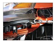
10. And finally, unbolt another bolt behind the factory horn using a 13mm socket coupled with a 10" extender, adjacent to the radiator. This is a bit tricky so take your time.
