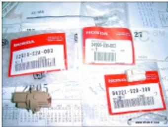
1 salvaged wire plug from any Honda/Acura with at least two pigtails (wires with terminal)
